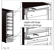
Check that the door sits level with the appliance. If not, the pivot plate offers some adjustment - loosen the screws you have just tightened and adjust the door as necessary.
