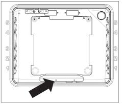
The oven burner is fixed in its cradle by a single clip that is placed on the left-hand side of the burner. Pull the clip further left, and with your other hand, lift the burner up holding from the thermocouple/spark plug holder.
